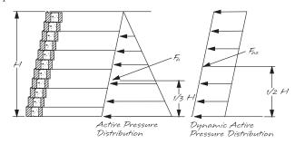
that the magnitude of the dynamic earth pressure should be applied to the wall as a rectangular distribution, radically changing the old theoretical inverted triangle method. The National Concrete Masonry Association (NCMA), FHWA and AASHTO have all adopted this methodology change.
