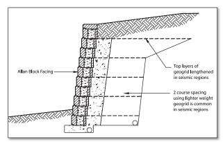
matic that Allan Block suggests using lightweight grids with a 2-course maximum spacing for all wall designs.
