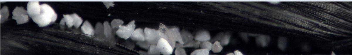
**Synonym for friction/adhesion:** microscopic interlock of soil particles with grid surface.
