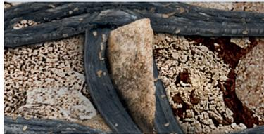
Penetration of stones and gravel through mesh openings, i.e. full interlock between rock components and grid.
