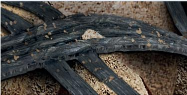
Interlock between soil particles and geogrid ribs due to surface texture.
