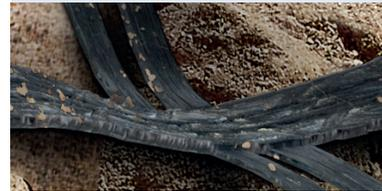
Ability of flexible geogrid to adapt to unevenness in soil during compaction.
