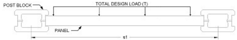
Figure 8: Panel Design Moment per Bond Beam
