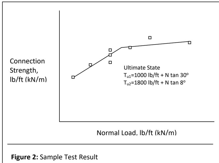
**Example:** Based on Figure 2: determine the Ultimate State Connection Strength for  $N = 863 \text{ lb/ft}$
