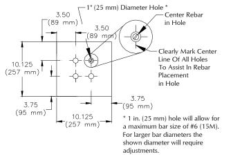
Figure 4 - Optional Alignment Plate
