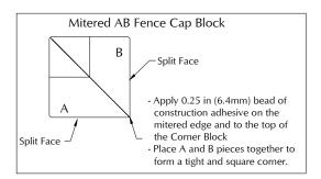
**Figure 5 – Miter Cutting Fence Corner Caps**
