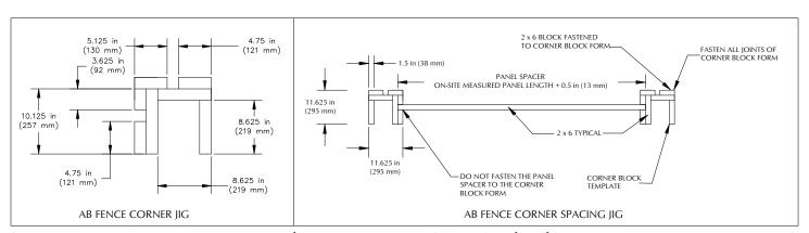
Figure 2 - AB Fence Corner Spacing Jig
