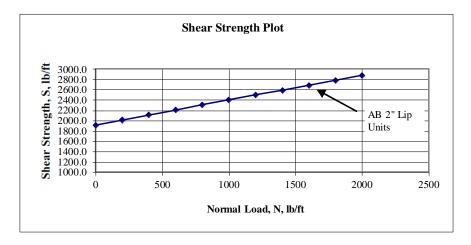
• ASTM D6638: Standard Test Method for Determining Strength Between Geosynthetic Reinforcement and Segmental Concrete Units
