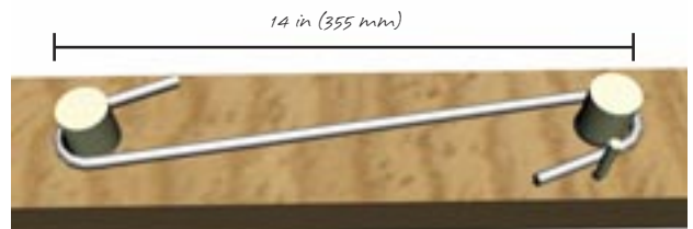
Figure 7: Stirrup Jig for Two-Course Bond Beam
