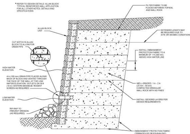
One benefit to this location was that the site soils consisted of sandy glacial till which allowed the use of existing soils, mixed with pulverized material from other areas of the site, in the infill area behind the wall facing. The free-draining property of this soil coupled with toe and heel drains, which were installed behind the wall, will allow it to handle any incidental water that makes its way behind the wall facing in accordance with Chapter 3 of the [Best Practices for SRW Walls](#).
