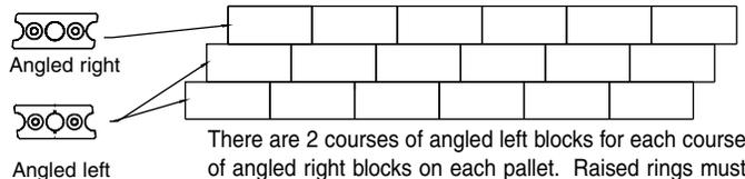
There are 2 courses of angled left blocks for each course of angled right blocks on each pallet. Raised rings must be facing up to determine left and right direction.
